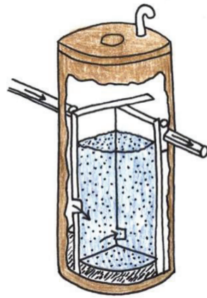
Figure 2.4: Illustration of a septic tank where effluent flow is redirected to another unit (Holmberg and Sundin 2005).
